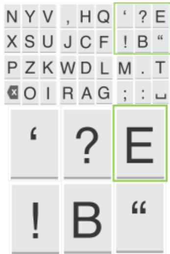
Figure 3. Sample layout of our early design. Users can select a character('E') by (1, top) selecting the corresponding group of characters (green circled), and (2, bottom) perform a second selection among previously selected characters only.
